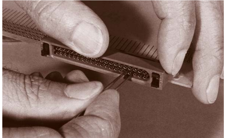
REMOVE DAMAGED CONTACT
