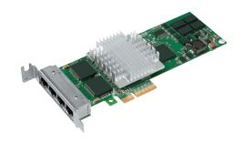
Server Adapter improves performance in multi-processor systems by balancing network loads across multiple central processing units (CPUs). Additionally, the Intel PRO/1000 PT Quad Port LP Server Adapter supports Intel® I/O Acceleration Technology (Intel® I/OAT)<sup>2</sup> for faster I/O processing on the new Quad-Core and Dual-Core Intel® Xeon® processor-based servers.
