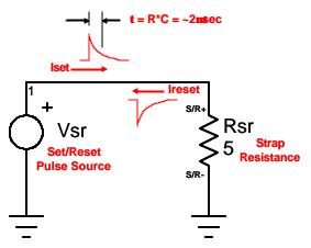
Figure 2 – A Simple Set/Reset Circuit
