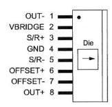
Arrow indicates direction of applied field that generates a positive output voltage after a SET pulse.
