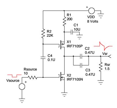
Figure 3 - Totem Pole Set/Reset Circuit for HMC1001
