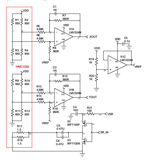
Figure 5 – 2-Axis Compass or Magnetometer
