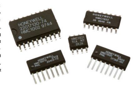
The HMC100x and HMC102x sensors utilize Honeywell's Anisotropic Magnetoresistive (AMR) technology that provides advantages over coil based magnetic sensors. They are extremely sensitive, low field, solid-state magnetic sensors designed to measure direction and magnitude of Earth's magnetic fields, from tens of micro-gauss to 6 gauss. Honeywell's Magnetic Sensors are among the most sensitive and reliable low-field sensors in the industry.
