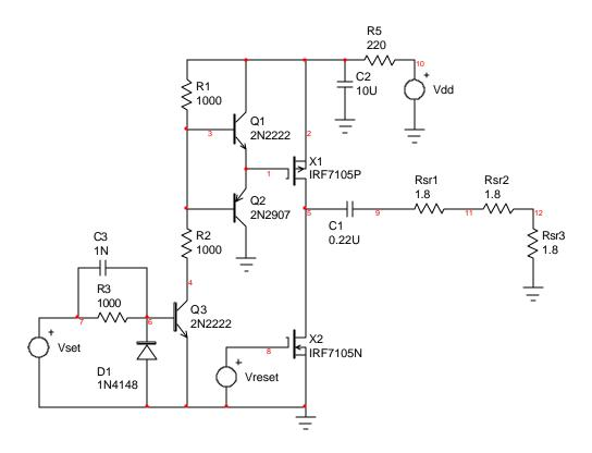
Figure 4 – Higher Voltage Set/Reset Circuit for HMC1001 & HMC1002
