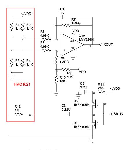
Figure 6 - Field Detector or Current Sensor
