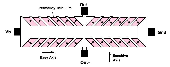
Figure 1 – Magneto-Resistive Wheatstone Bridge Elements
