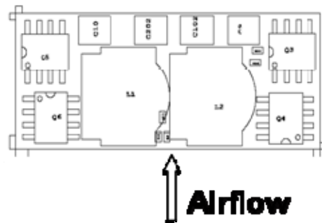
Figure 55. Airflow direction for thermal testing.
