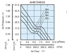
■ P & Q CURVE (AT RATED VOLTAGE)
