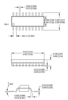
**20X**, 20-lead, 4.4 mm Wide, Plastic Thin Shrink Small Outline (TSSOP) Dimensions in Millimeters and (Inches)\*
