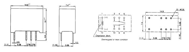
NAL-D type (double winding latching type)
