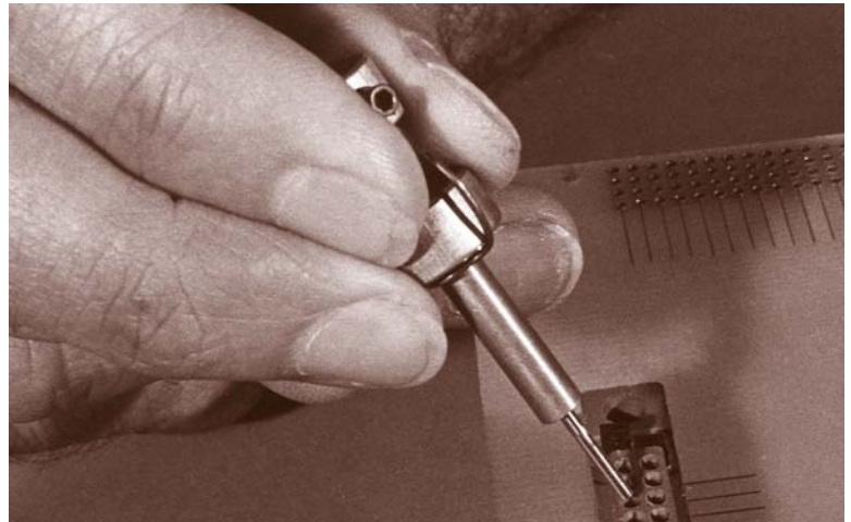
INSERT EXTRACTION TOOL WITH PLUNGER RETRACTED
