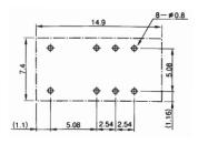
NAL-D (Double winding latching type)
