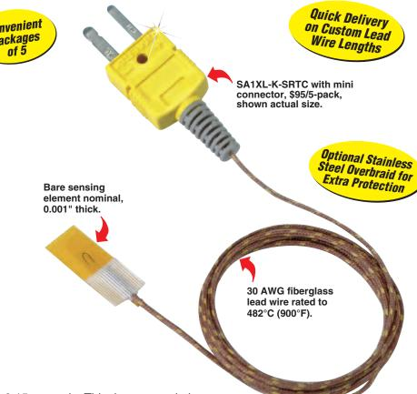
0.15 seconds. This thermocouple is constructed using a Polyimide/ fiberglass-junction insulation along with a fiberglass-insulated lead wire. The SA1XL can be used as a self-adhering thermocouple for temperatures up to 260°C (500°F) or it can be cemented in place for use at temperatures up to 315°C (600°F).
