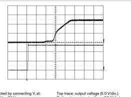
Start-up enabled by connecting  $V_{\scriptscriptstyle I}$  at:  $T_{ref} = +25$ °C,  $V_1 = 27$  V,  $I_0 = 1$  A resistive load.
