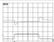
Output voltage response to load current step-change (0.5-1.5-0.5 A) at: Bottom trace: load current (1 A/div.).  $T_{ref} = +25^{\circ}\text{C}, \ V_{I} = 27 \text{ V}.$  Time scale: (0.1 ms/div.).
