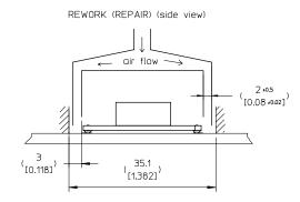
Recommended design of a hot air rework nozzle for manual removal and re-mounting: double wall design directs air flow to solder bump edges only.
