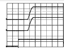
Start-up enabled by connecting  $V_i$  at:  $T_{ref} = +25^{\circ}C$ ,  $V_i = 27$  V,  $I_0 1 = 0.62$  A,  $I_0 2 = 0.62$  A resistive load.
