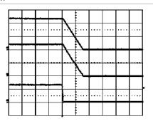
Shut-down enabled by disconnecting V<sub>I</sub> at:  $T_{ref} = +25^{\circ}C$ , V<sub>I</sub> = 27 V,  $I_{O}1 = 0.62$  A,  $I_{O}2 = 0.62$  A resistive load.
