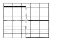
Shut-down enabled by disconnecting  $V_{\scriptscriptstyle I}$  at:  $T_{ref} = +25$ °C,  $V_I = 27$  V,  $I_O = 2$  A resistive load.
