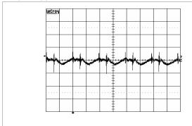
Output voltage ripple at:  $T_{ref} = +25$ °C,  $V_{l} = 27$  V,  $I_{O} = 2$  A resistive load.
