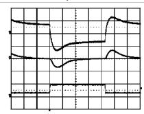
Output voltage response to load current step-change, output 1 (0.16-0.47-0.16 A) at:  $T_{ref}$  =+25°C,  $V_I$  = 27 V  $I_O$ 2 = 0.62 A.
