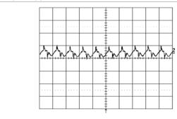
Output voltage ripple at:  $T_{ref} = +25^{\circ}C$ ,  $V_{I} = 27 V$ ,  $T_{ref} = +25^{\circ}C$ ,  $V_1 = \angle i v$ ,  $I_0 = 2$  A resistive load.
