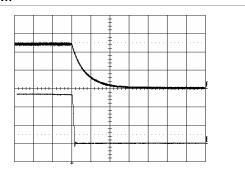
Shut-down enabled by disconnecting  $V_{\scriptscriptstyle I}$  at:  $T_{ref} = +25$ °C,  $V_I = 27$  V,  $I_O = 1$  A resistive load.
