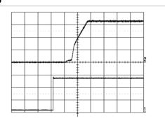
Start-up enabled by connecting  $V_i$  at:  $T_{ref} = +25$ °C,  $V_1 = 27$  V,  $I_0 = 2$  A resistive load.
