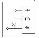
The products are fitted with a remote control function referenced to the primary negative input connection (- In), and have positive logic. The RC function allows the converter to be turned on/off by an external device like a semiconductor or mechanical switch.
