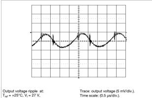
$T_{ref} = +25$ °C,  $V_I = 27$  V  $I_O = 1$  A resistive load.
