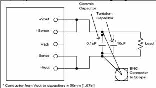
Output ripple and noise test setup
