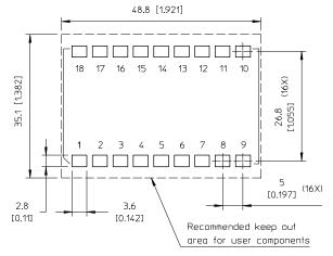
The recommended footprint (see previous page) is optimised for the solder bump design. However, the standard PKF footprint will also accompdate this solder bump design. The only differences is the solder pad width (2.8 versus 2.3 mm) and the c-c distance between the two rows of solder lands (26.8 versus 26.6 mm).
