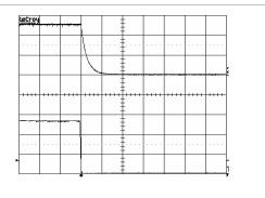
Shut-down enabled by disconnecting V<sub>i</sub> at:  $T_{ref}$  = +25°C, V<sub>i</sub> = 27 V,  $I_O$  = 2 A resistive load.
