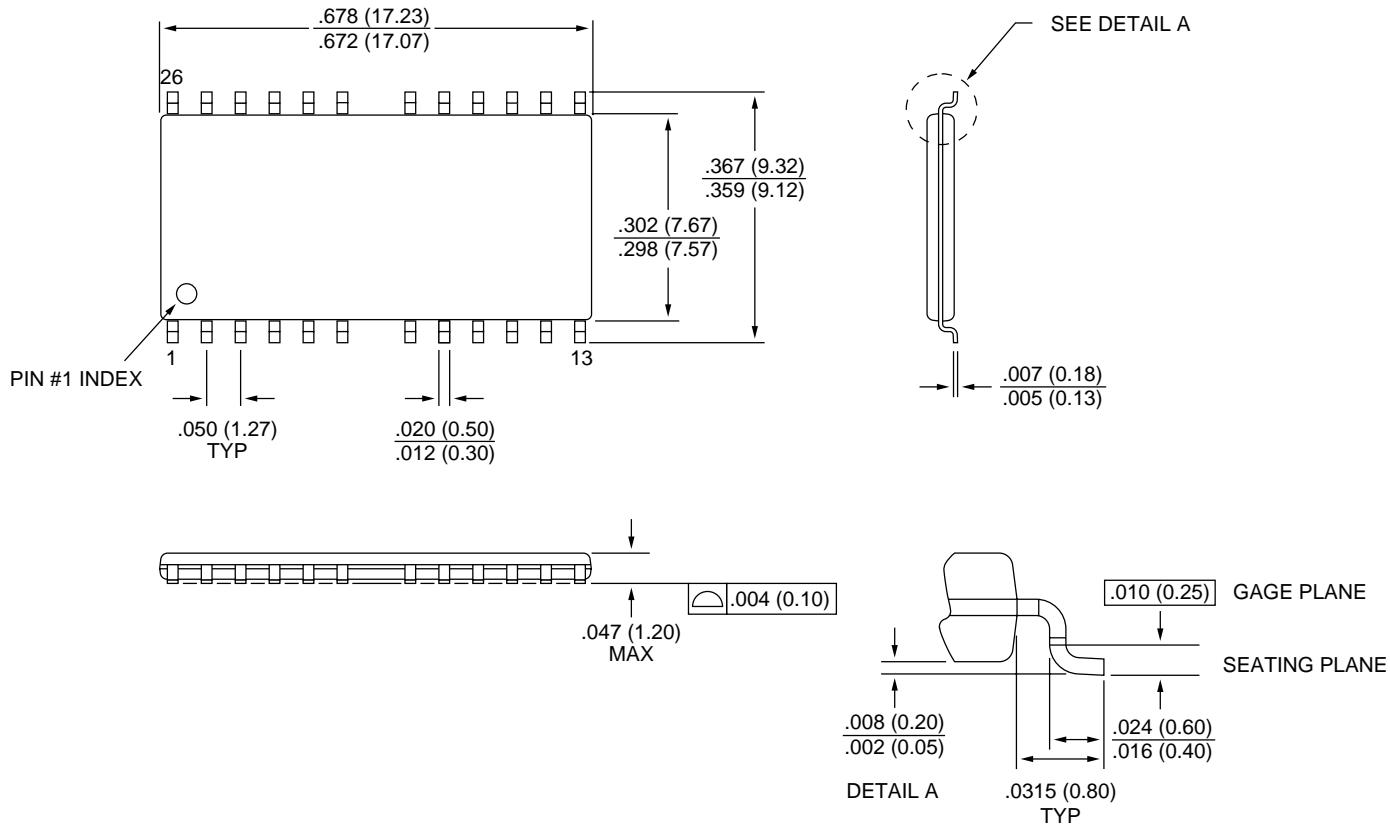
**NOTE:** 1. All dimensions in inches (millimeters)  $\frac{\text{MAX}}{\text{MIN}}$  or typical where noted.
