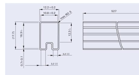
Tube for THT version 25 relays per tube 1'000 relays per box
