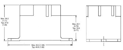
Note: Allow air circulation within the sealed type G8PT by removing the ventilation nib from the cover after soldering and cleaning is complete.
