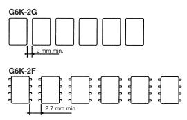
Two or more Relays may be mounted as closely as desired with the short sides of the Relays facing each other.
