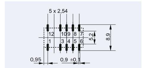
Note: Solder pad for pin 6 and 7 only for latching with 2 coils
