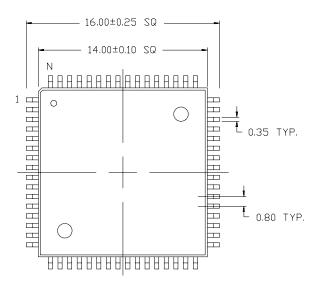
DIMENSIONS IN MILLIMETERS LEAD COPLANARITY 0.102 MAX.
