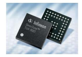
O M N I T U N E <sup>™</sup> T U A 9 0 0 1 is a highly integrated CMOS Direct Conversion Receiver (DCR), supports DVB-H/T and CMMB for mobile and portable multimedia solutions. OMNITUNE™ TUA 9001 covers VHF, UHF as well as L-bands for Europe and US frequency ranges. It can be operated with either a single or dual supply with a power consumption as low as 18mW at 10% duty cycle operation in DVB-H mode and 190mW in DVB-T mode.
