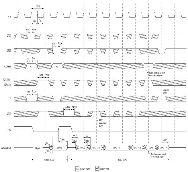
Note: 17. On this diagram, when  $\overline{CE}$  is LOW,  $\overline{CE}_1$  is LOW,  $\overline{CE}_2$  is HIGH and  $\overline{CE}_3$  is LOW. When  $\overline{CE}$  is HIGH,  $\overline{CE}_1$  is HIGH or  $\overline{CE}_2$  is LOW or  $\overline{\overline{CE}}_3$  is HIGH.
