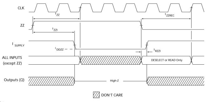
21. Device must be deselected when entering ZZ mode. See Cycle Descriptions table for all possible signal conditions to deselect the device. 22. DQs are in High-Z when exiting ZZ sleep mode.
