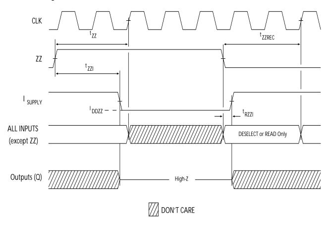
21. Device must be deselected when entering ZZ mode. See Cycle Descriptions table for all possible signal conditions to deselect the device. 22. DQs are in high-Z when exiting ZZ sleep mode.
