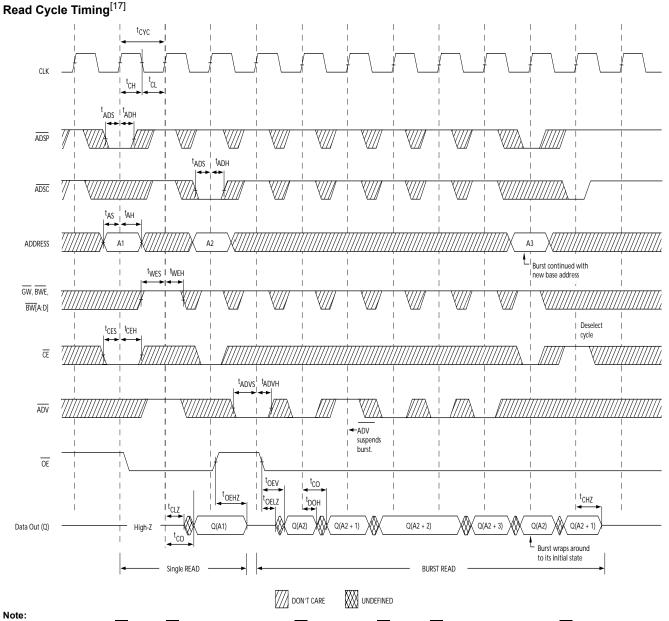
17. On this diagram, when  $\overline{CE}$  is LOW,  $\overline{CE}_1$  is LOW,  $CE_2$  is HIGH and  $\overline{CE}_3$  is LOW. When  $\overline{CE}$  is HIGH,  $\overline{CE}_1$  is HIGH or  $CE_2$  is LOW or  $\overline{CE}_3$  is HIGH.
