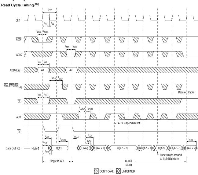
Note: 16. On this diagram, when  $\overline{\text{CE}}$  is LOW,  $\overline{\text{CE}}_1$  is LOW,  $\overline{\text{CE}}_2$  is HIGH and  $\overline{\text{CE}}_3$  is LOW. When  $\overline{\text{CE}}$  is HIGH,  $\overline{\text{CE}}_1$  is HIGH or  $\overline{\text{CE}}_2$  is LOW or  $\overline{\text{CE}}_3$  is HIGH.
