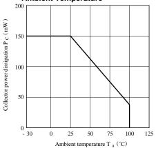
Fig. 2 Diode Power Dissipation vs. Ambient Temperature
