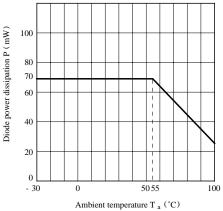
Fig. 4 Power Dissipation vs. Ambient Temperature
