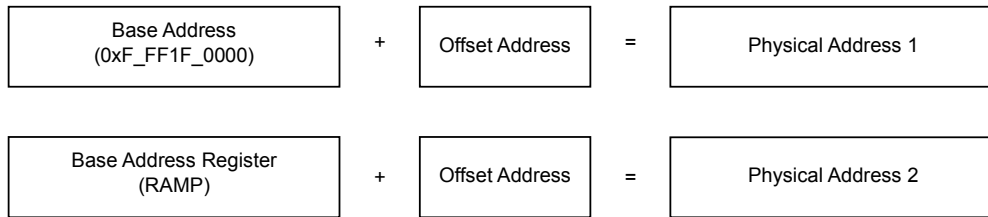
Figure 4.2.1 Generating Physical Address for a Internal Register
