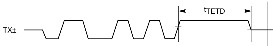
Figure 55 10 Mbps Transmit (TX±) Timing Diagram
