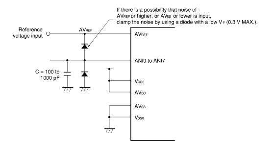
Figure 11-9. Processing Analog Input Pin
