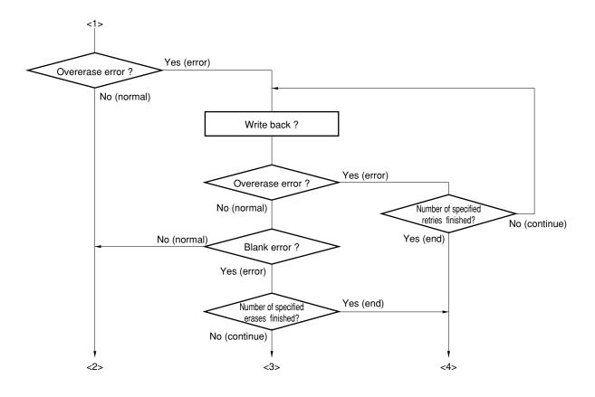
Figure 18-16. Self Programming Flowchart (2/2)
