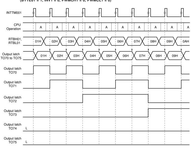
(a) 6 bits  $\times$  1 channel, inverted output disabled, no PWM modulation (BYTE01 = 1, INV1 = 0, PWMCH1 = 0, PWMCL1 = 0)
