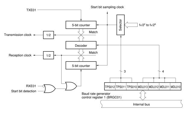
RemarkTXE01: Bit 7 of asynchronous serial interface mode register 1 (ASIM01)RXE01: Bit 6 of asynchronous serial interface mode register 1 (ASIM01)
