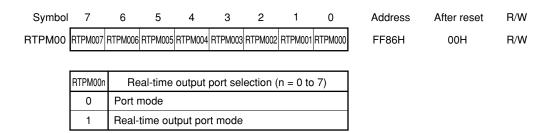
Caution When using a port as a real-time output port, set the port in the output mode (by clearing the corresponding bit of port mode register 3 (PM3) to 0).
