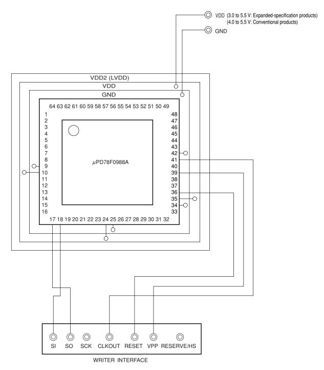
Figure 18-12. Wiring Example for Flash Writing Adapter with UART (UART00)
