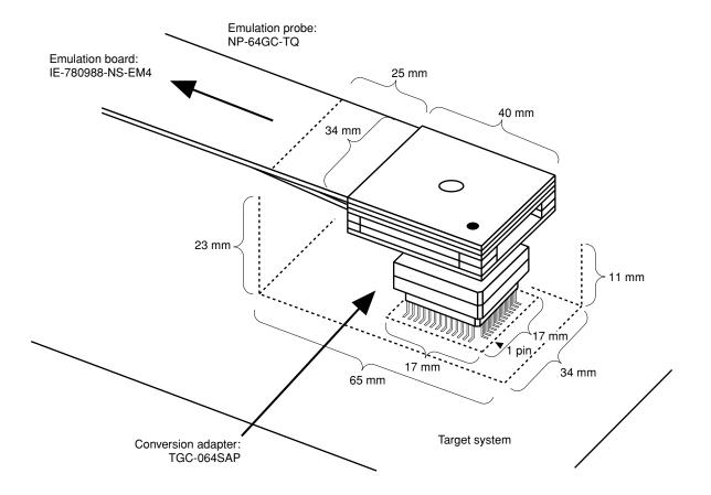
Figure B-4. Connection Condition of Target System (1)
