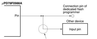
If the signal output by the  $\mu$ PD78F0988A affects another device in the flash memory programming mode, isolate the signals of the other device.
