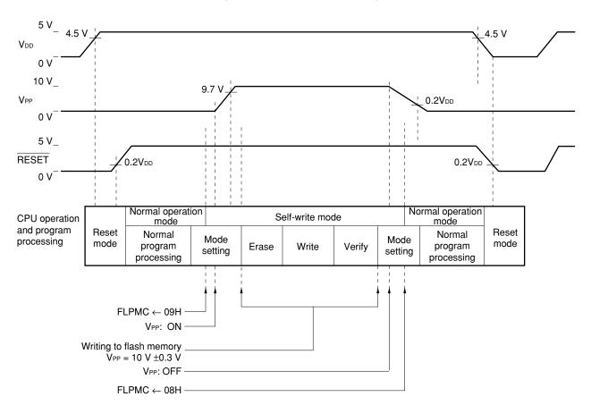
Figure 18-17. Self-Write Timing
