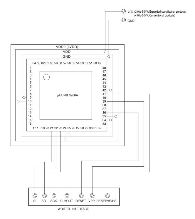
Figure 18-13. Wiring Example for Flash Writing Adapter with Pseudo 3-Wire Serial I/O
