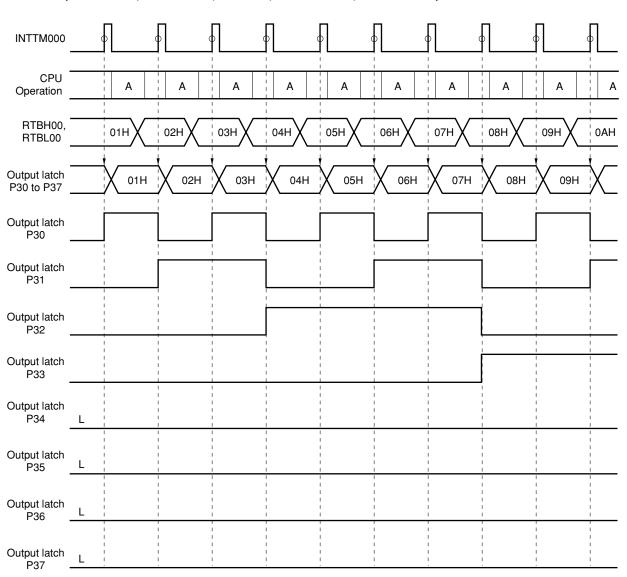
(a) 8 bits  $\times$  1 channel, inverted output disabled, no PWM modulation (EXTR00 = 0, BYTE00 = 1, INV0 = 0, PWMCH0 = 0, PWMCL0 = 0)
