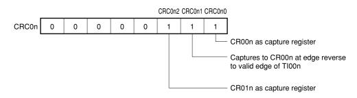
**Remarks 1.** 0/1: Setting 0 or 1 allows another function to be used simultaneously with pulse width measurement. See **Figures 6-3** and **6-4** for details.
