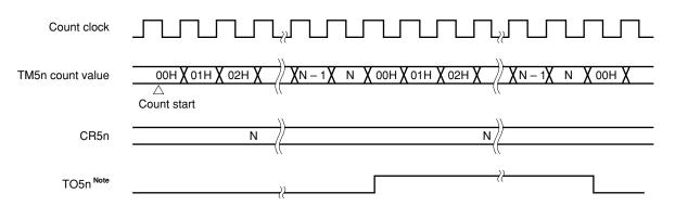
**Note** The initial value of TO5n output can be set with bits 2 and 3 (LVR5n and LVS5n) of 8-bit timer mode control register 5n (TMC5n).
