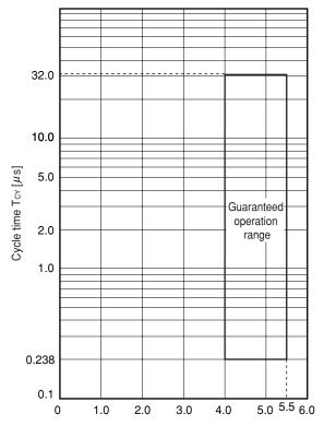
TCY VS VDD (System clock operation)
