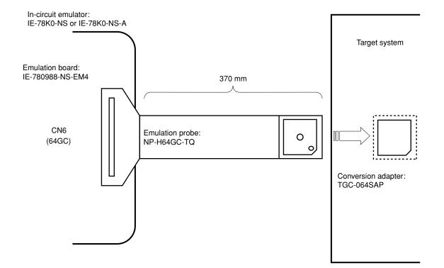
Figure B-2. Distance Between In-Circuit Emulator and Conversion Socket or Conversion Adapter (2)
