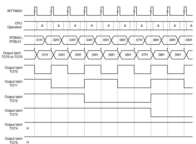
Figure 10-12. Real-Time Output Port Operation Timing Example (6 Bits  $\times$  1) (2/3)
