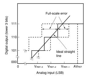
Figure 11-21. Integral Linearity Error
