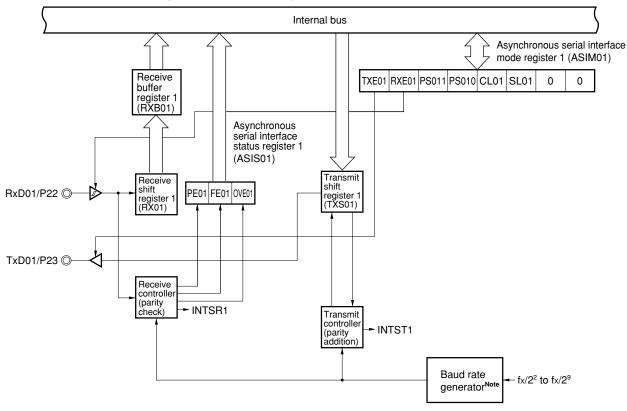
Figure 12-3. Block Diagram of Serial Interface UART01
