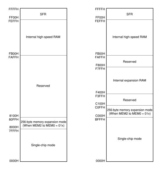
Figure 15-1. Memory Map When External Device Expansion Function Used (3/3)
