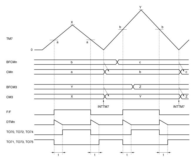
Figure 8-4. TM7 Operation Timing (Basic Operation)
