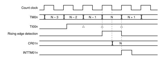
Figure 6-22. CR01n Capture Operation with Rising Edge Specified
