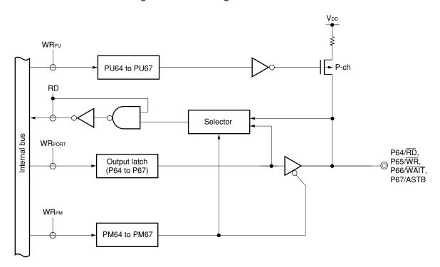
Figure 4-9. Block Diagram of P64 to P67
