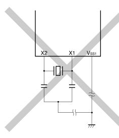
(c) Wiring near high fluctuating current
