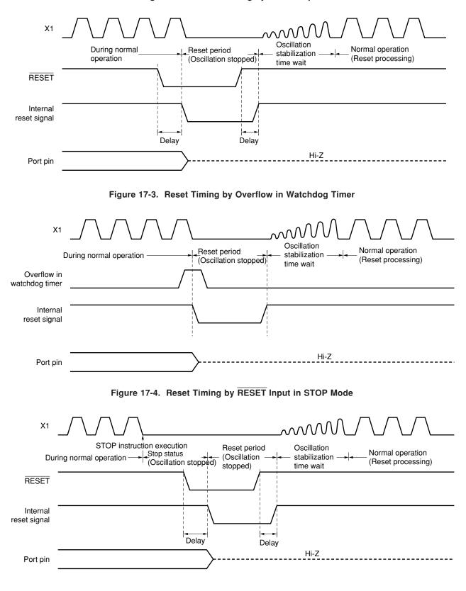
Figure 17-2. Reset Timing by RESET Input
