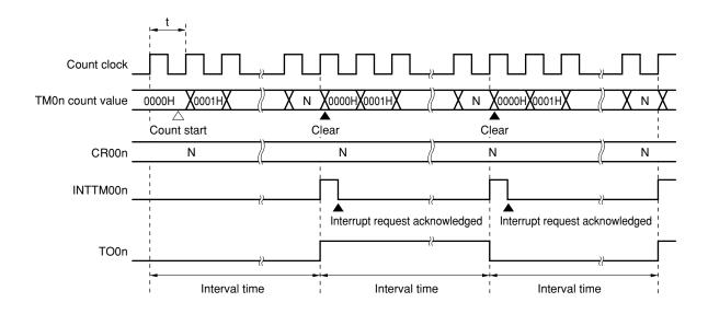
**Remarks 1.** Interval time =  $(N + 1) \times t$ : N = 0001H to FFFFH **2.** n = 0, 1
