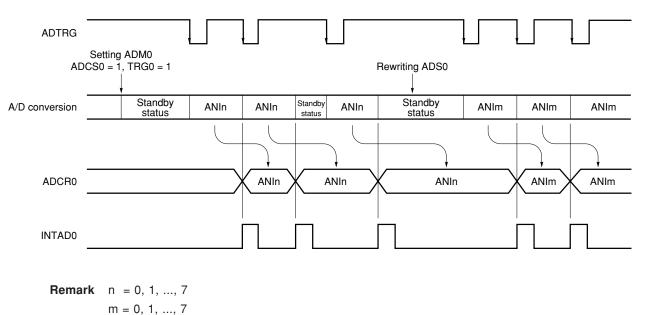
Figure 11-6. A/D Conversion by Hardware Start (with Falling Edge Specified)
