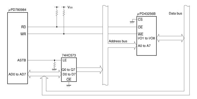
Figure 15-9. Example of Connecting  $\mu$ PD780984 and Memory
