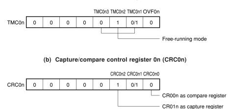
**Remarks 1.** 0/1: Setting 0 or 1 allows another function to be used simultaneously with pulse width measurement. See **Figures 6-3** to **6-6** for details.
