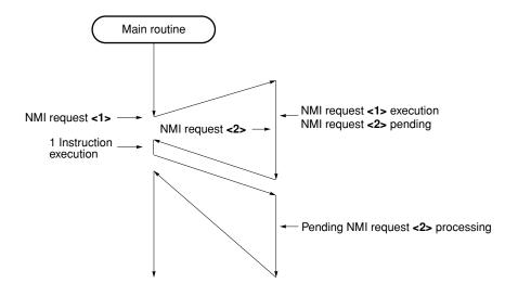
(b) If two new non-maskable interrupt requests are generated while non-maskable interrupt service program is being executed
