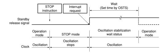
**Remark** The dotted lines indicate the case when the interrupt request that has released the standby mode is acknowledged.
