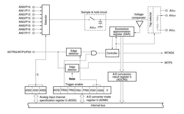
Figure 11-1. A/D Converter Block Diagram
