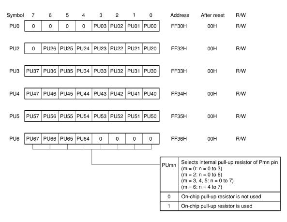
Figure 4-11. Format of Pull-up Resistor Option Register
