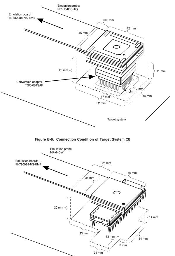
Figure B-5. Connection Condition of Target System (2)
