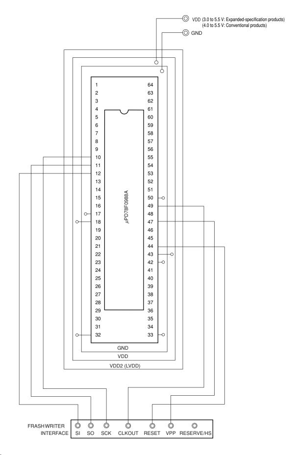
Figure 18-11. Wiring Example for Flash Writing Adapter with 3-Wire Serial I/O (SIO3) with Handshake
