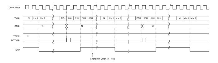
(c) If value of CR5n is changed from N to M within 2 clocks (00H, 01H) immediately after TM5n overflows
