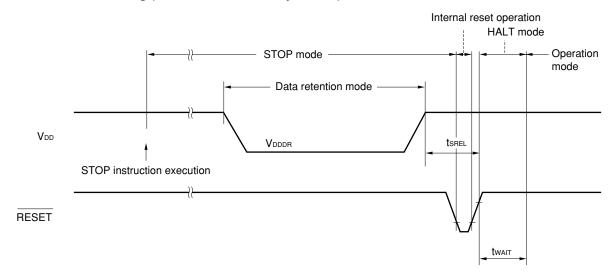
Data Retention Timing (Standby Release Signal: STOP Mode Release by Interrupt Request Signal)
