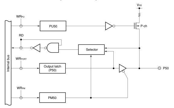
Figure 4-7. Block Diagram of P50
