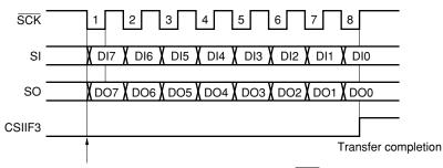
Figure 13-3. Timing of 3-Wire Serial I/O Mode
