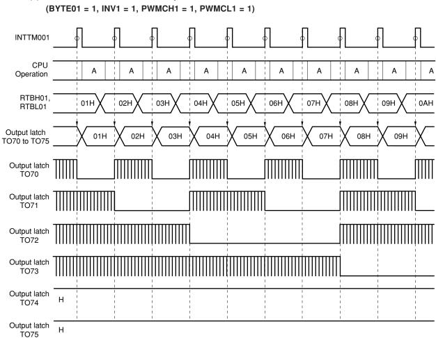
(c) 6 bits  $\times$  1 channel, inverted output enabled, PWM modulation (BYTE01 = 1, INV1 = 1, PWMCH1 = 1, PWMCI 1 = 1)
