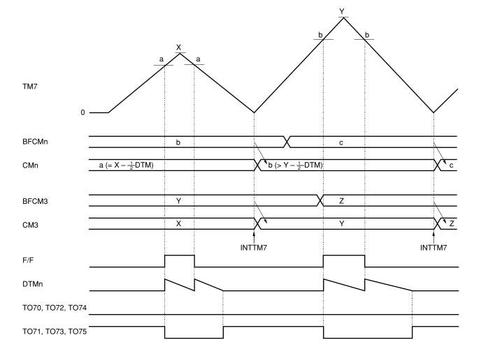
Figure 8-7. TM7 Operation Timing (CMn (BFCMn) = CM3 – 1/2DTM, CMn (BFCMn) > CM3 – 1/2DTM)
