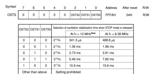
Figure 9-4. Format of Oscillation Stabilization Time Select Register
