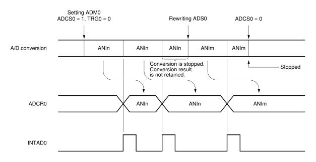
Figure 11-7. A/D Conversion by Software Start
