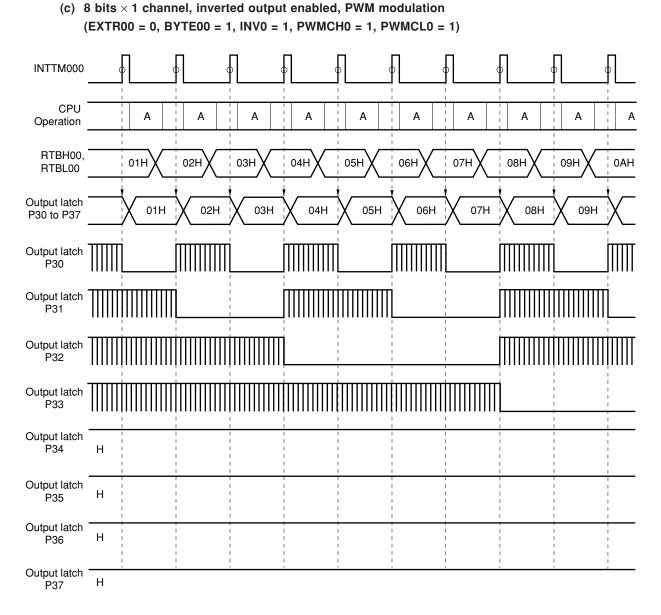
Figure 10-11. Real-Time Output Port Operation Timing Example (8 Bits  $\times$  1) (3/3)
