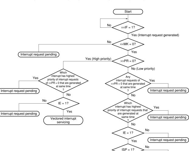
Figure 14-11. Interrupt Request Acknowledgement Program Algorithm
