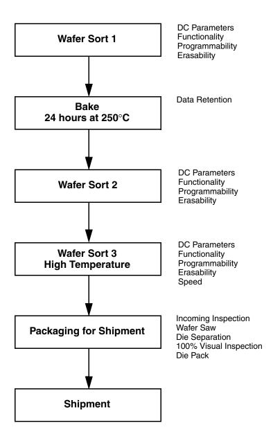
Figure 1. AMD KGD Product Test Flow
