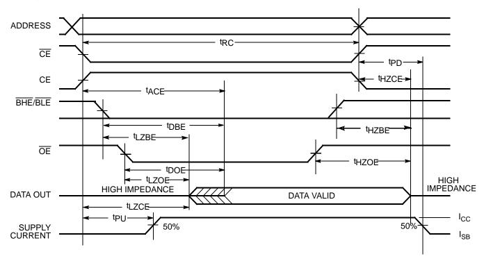
20. <u>The</u> device is continuously selected. OE,  $\overline{CE}_1 = V_{IL}$ ,  $\overline{BHE}$  and/or  $\overline{BLE} = V_{IL}$ , and  $CE_2 = V_{IH}$ .
