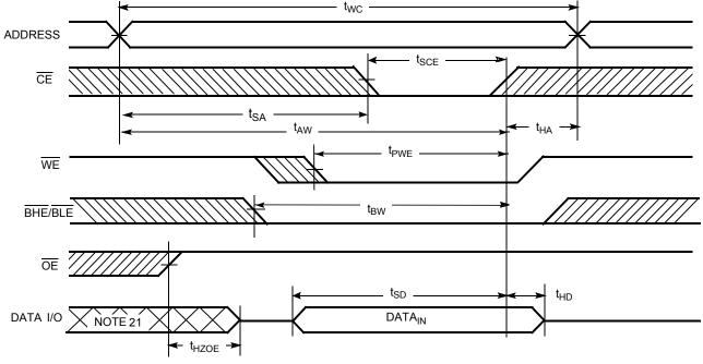
Notes: 19. Data I/O is high impedance if  $\overline{OE} = V_{IH}$ . 20. If  $\overline{CE}$  goes HIGH simultaneously with  $\overline{WE} = V_{IH}$ , the output remains in a high-impedance state. 21. During this period, the I/Os are in output state and input signals should not be applied.
