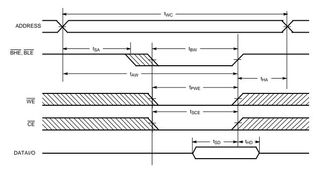
**Notes:** 16. Data I/O is high-impedance if  $\overline{OE}$  or  $\overline{BHE}$  and/or  $\overline{BLE} = V_{IH}$ . 17. If  $\overline{CE}_1$  goes HIGH simultaneously with WE going HIGH, the output remains in a high-impedance state. 18.  $\overline{CE}$  is a shorthand combination of both  $\overline{CE}_1$  and  $CE_2$  combined. It is active LOW.
