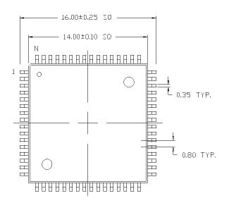
DIMENSIONS IN MILLIMETERS LEAD COPLANARITY 0,102 MAX.
