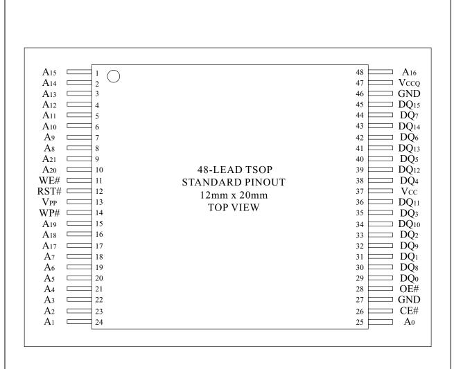
Figure 1. 48-Lead TSOP (Normal Bend) Pinout
