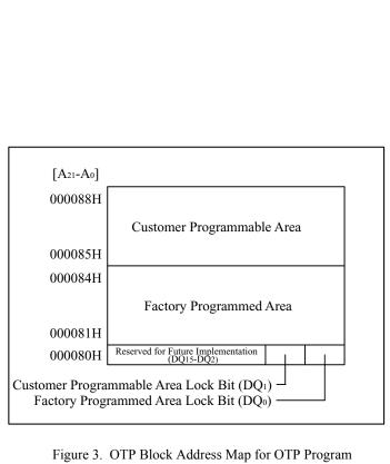
Figure 3. OTP Block Address Map for OTP Program (The area outside 80H~88H cannot be used.)
