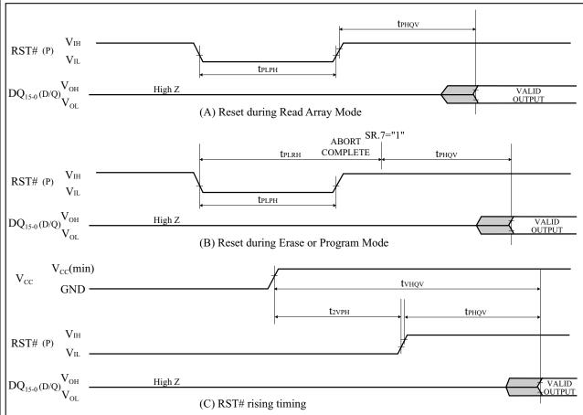
Figure 10. AC Waveform for Reset Operations
