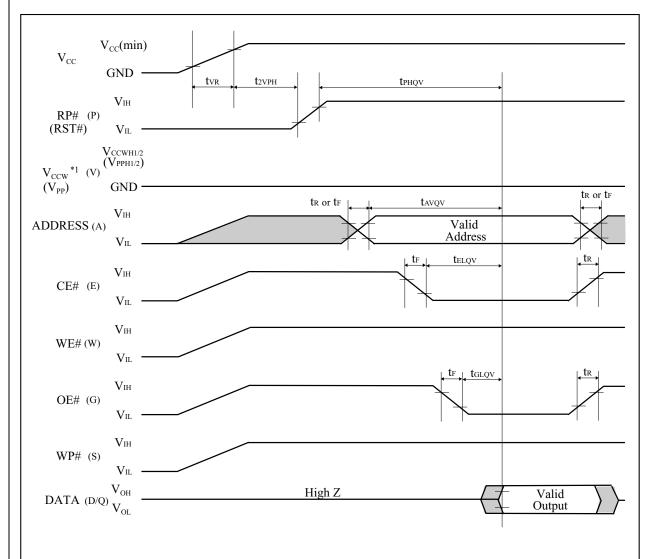
\*1 To prevent the unwanted writes, system designers should consider the design, which applies  $V_{CCW}$  ( $V_{PP}$ ) to 0V during read operations and  $V_{CCWH1/2}$  ( $V_{PPH1/2}$ ) during write or erase operations. See the application note AP-007-SW-E for details.
