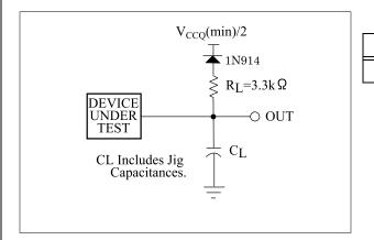
Figure 6. Transient Equivalent Testing Load Circuit
