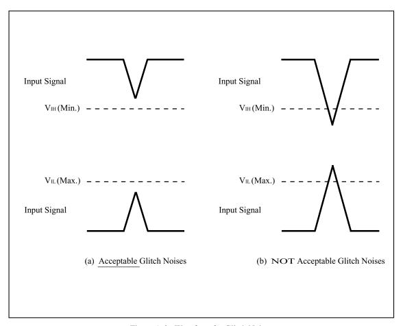
Figure A-2. Waveform for Glitch Noises
