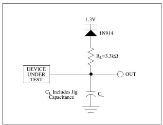
Figure 15. Transient Equivalent Testing Load Circuit
