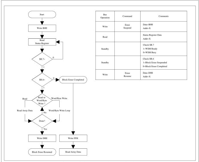
Figure 9. Block Erase Suspend/Resume Flowchart
