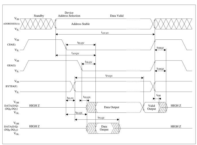
Figure 17. BYTE# timing Waveform
