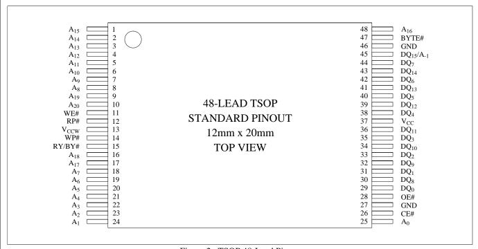
Figure 2. TSOP 48-Lead Pinout
