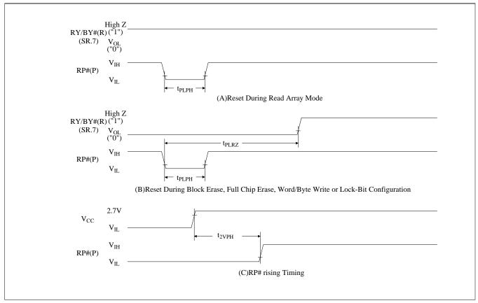
Figure 20. AC Waveform for Reset Operation
