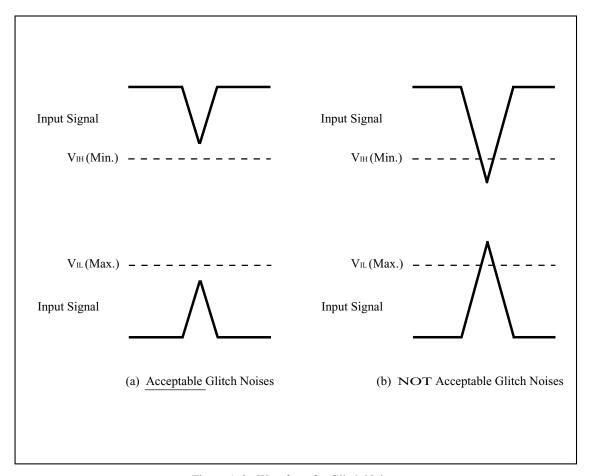
Figure A-2. Waveform for Glitch Noises
