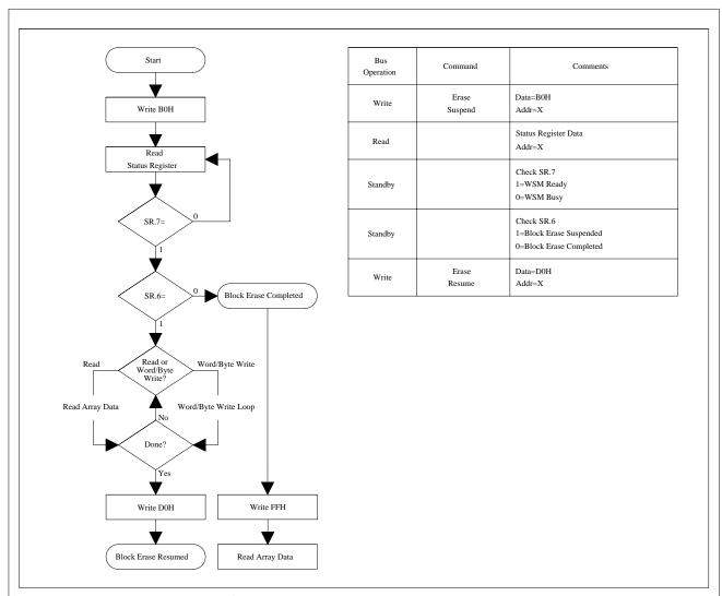
Figure 7. Block Erase Suspend/Resume Flowchart
