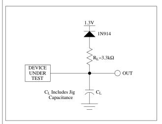
Figure 10. Transient Equivalent Testing Load Circuit
