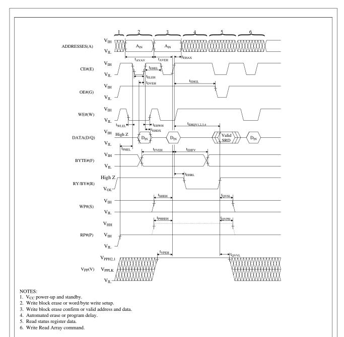
Figure 14. AC Waveform for CE#-Controlled Write Operations
