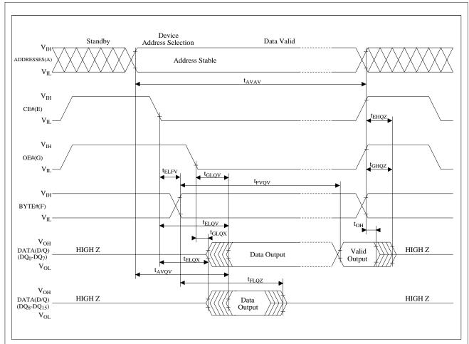
Figure 12. BYTE# timing Waveform
