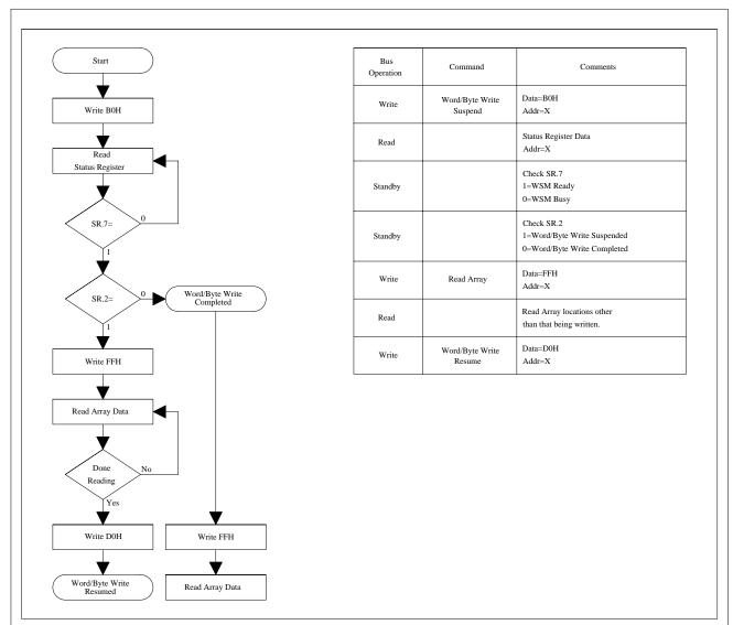
Figure 8. Word/Byte Write Suspend/Resume Flowchart
