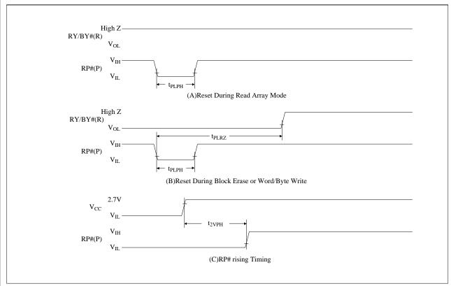
Figure 15. AC Waveform for Reset Operation
