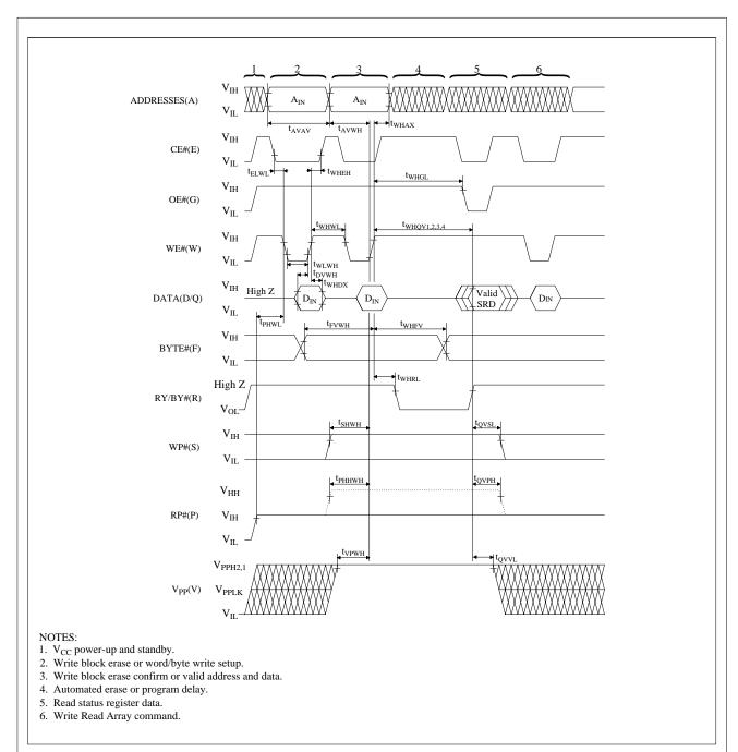
Figure 13. AC Waveform for WE#-Controlled Write Operations
