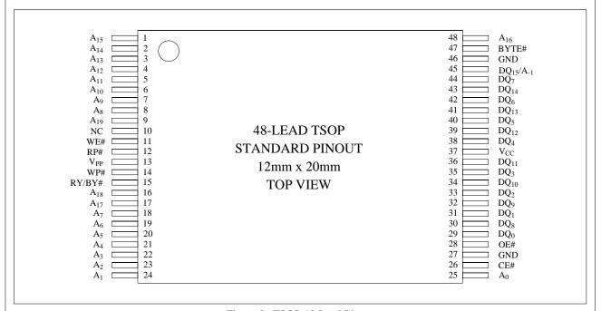
Figure 2. TSOP 48-Lead Pinout
