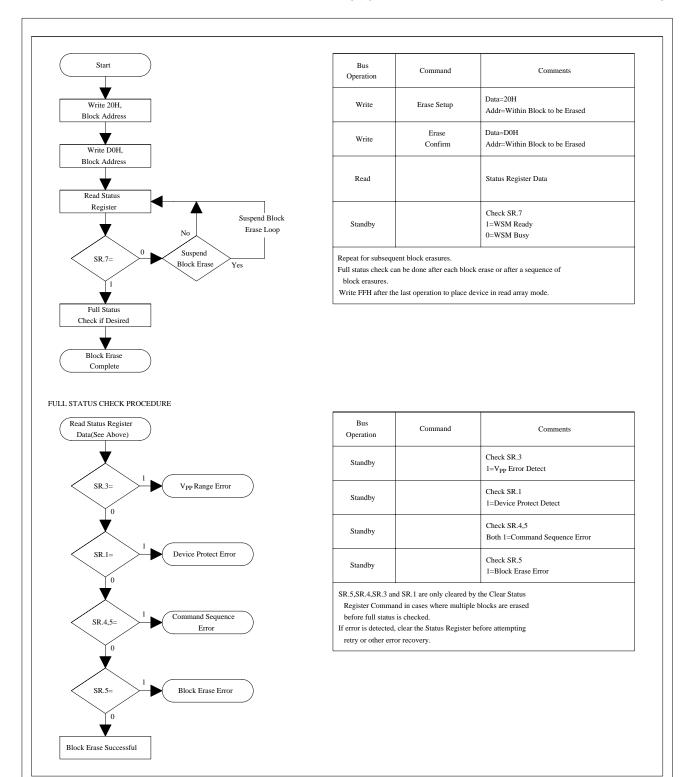
Figure 5. Automated Block Erase Flowchart
