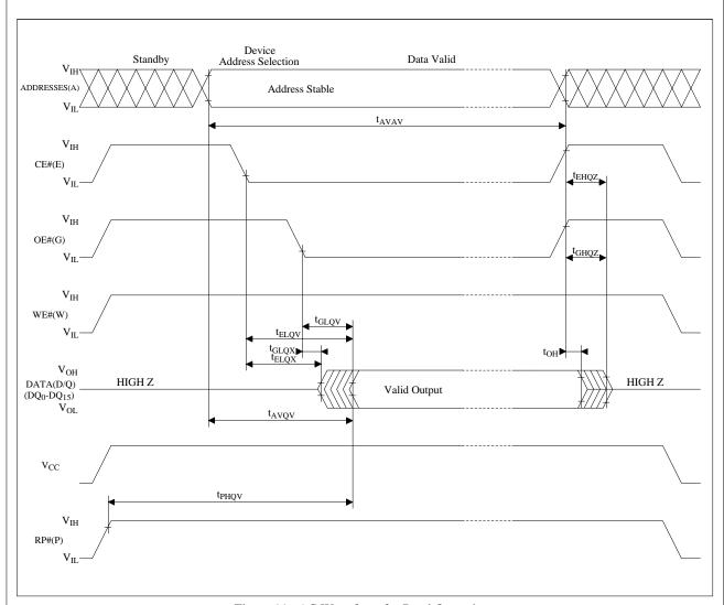
Figure 11. AC Waveform for Read Operations
