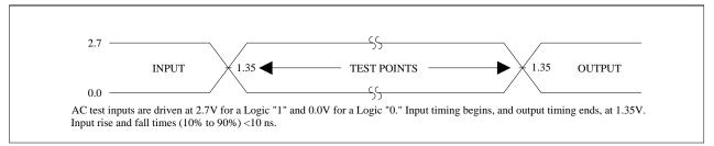
Figure 9. Transient Input/Output Reference Waveform for  $V_{CC}$ =2.7V-3.6V
