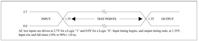
Figure 12. Transient Input/Output Reference Waveform for  $V_{CC}$ =2.7V-3.6V
