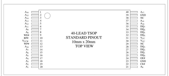
Figure 2. TSOP 40-Lead Pinout
