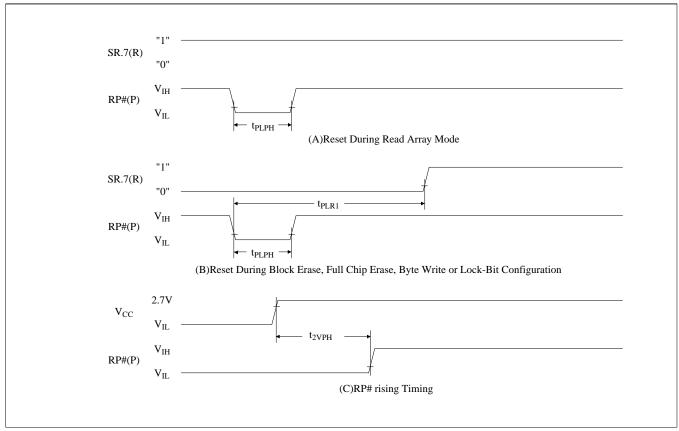
Figure 17. AC Waveform for Reset Operation
