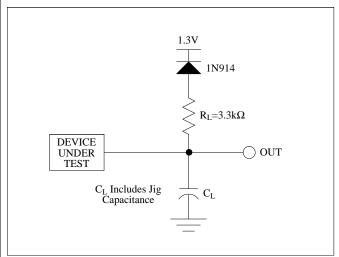
Figure 13. Transient Equivalent Testing Load Circuit
