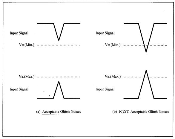
Figure A-2. Waveform for Glitch Noises
