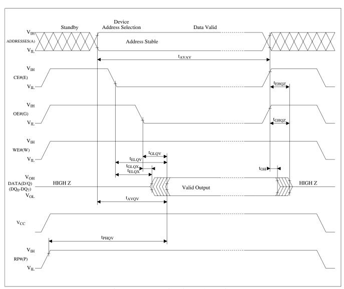
Figure 14. AC Waveform for Read Operations
