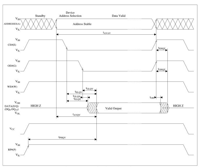
Figure 16. AC Waveform for Read Operations
