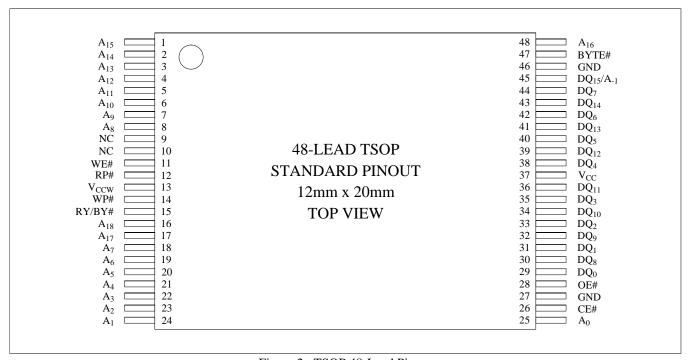
Figure 2. TSOP 48-Lead Pinout
