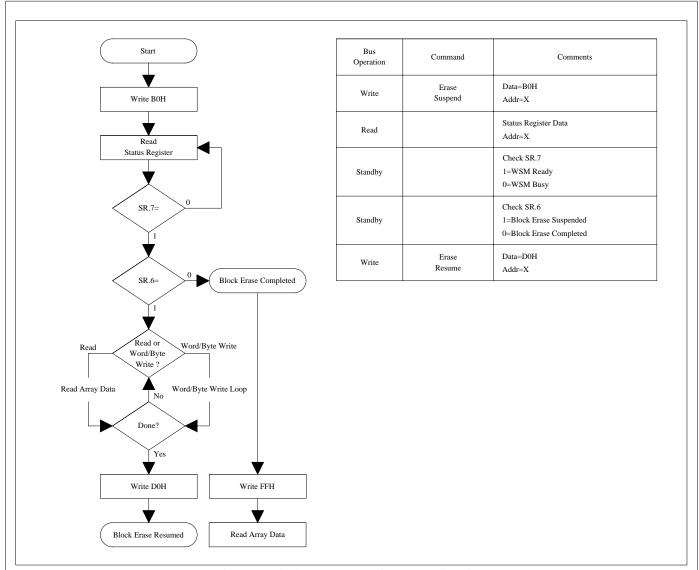
Figure 9. Block Erase Suspend/Resume Flowchart
