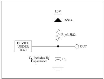
Figure 15. Transient Equivalent Testing Load Circuit
