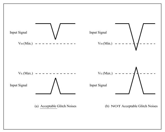
Figure A-2. Waveform for Glitch Noises
