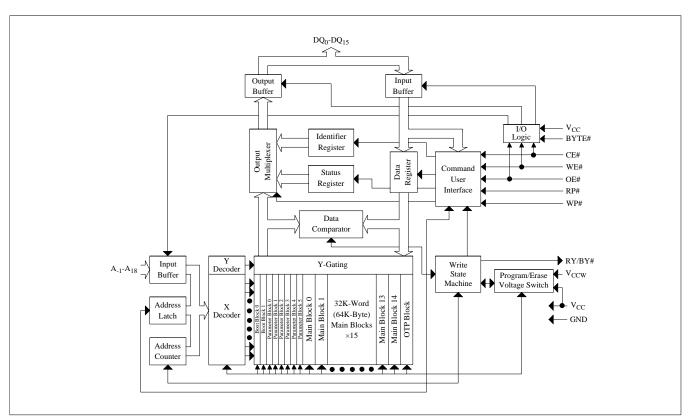
Figure 1. Block Diagram
