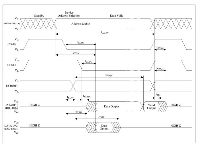
Figure 17. BYTE# timing Waveform
