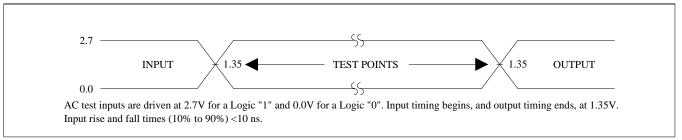
Figure 14. Transient Input/Output Reference Waveform for  $V_{CC}$ =2.7V-3.6V
