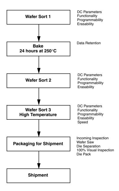
Figure 1. AMD KGD Product Test Flow
