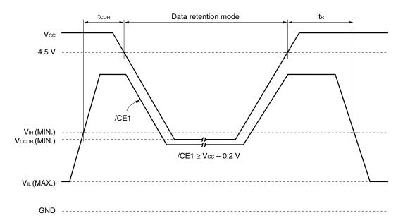
**Remark** On the data retention mode by controlling /CE1, the input level of CE2 must be CE2  $\geq$  Vcc - 0.2 V or CE2  $\leq$  0.2 V. The other pins (Address, I/O, /WE) can be in high impedance state.
