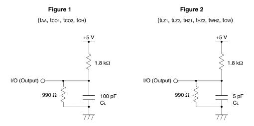
Remark C<sub>L</sub> includes capacitance of the probe and jig, and stray capacitance.
