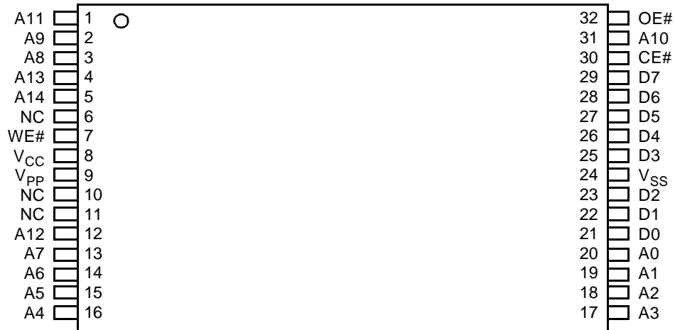
32-Pin TSOP—Standard Pinout
