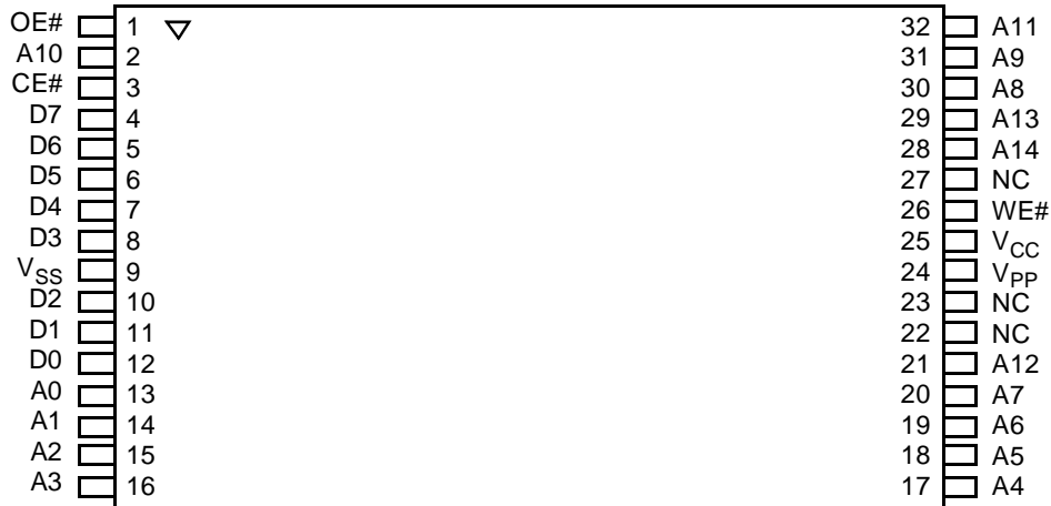
32-Pin TSOP—Reverse Pinout
