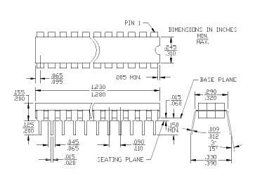
24-Lead (300-Mil) CerDIP D14 MIL-STD-1835 D- 9Config.A
