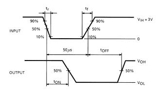
Note 1: Pulse Width 50  $\mu s$ , duty cycle 10%
