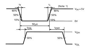
Note 1: Pulse width 50  $\mu$ s, duty cycle 10% Output impedance 50  $\Omega$ ,  $t_\Gamma \le 5$  ns,  $t_f \le 10$  ns
