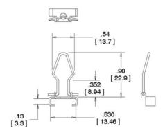
Plastic Connector Mounted to Front of Panel
