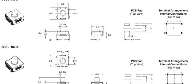
**Note:** Unless otherwise specified, a tolerance of  $\pm 0.2$  mm applies to all dimensions.
