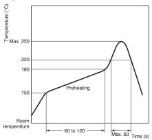
Note: The above heating curve applies if the PCB thickness is 1.6 mm.
