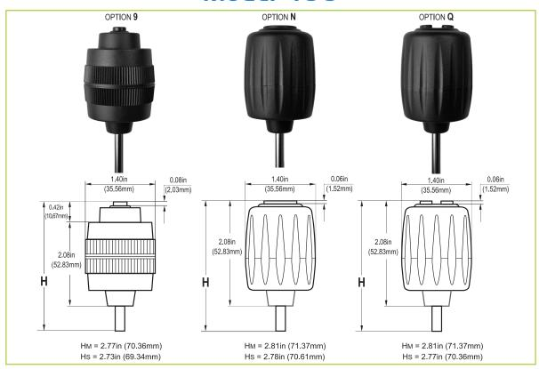
NOTES: HM = height above the housing (H) for Miniature Joysticks Hs = height above the housing (H) for Standard Joysticks
