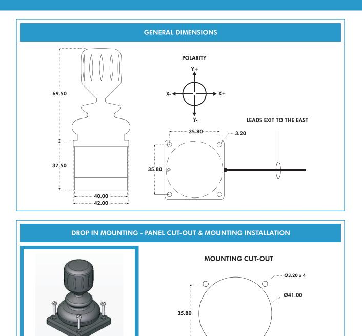
Note: The dimensions shown are for a generic 9000 Series with the third axis R type handle. For specific dimensions of this or any other configuration please refer to Apem.
