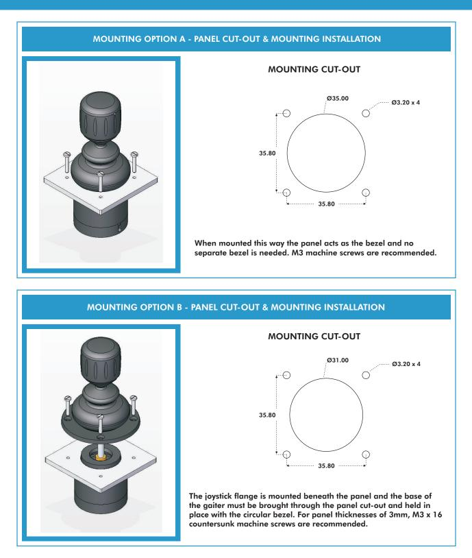
Note: When sub panel mounting, great care should be taken not to damage the gaiter, or any of the mechanism under the gaiter. All panel cut-outs should be free from sharp edges and swarf that may damage the gaiter.
