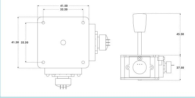
Note: The dimensions shown are for a generic two axes 5000 Series with the F type handle. For specific dimensions of this or any other configuration please refer to Apem.
