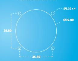
The joystick is dropped into the panel cut-out. For panel thickness of <3mm, M3 x 16 countersunk machine screws are recommended.lllustration (left) shows the square bezel option, a circular bezel is also available.
