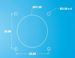
The joystick flange is mounted beneath the panel and the base of the gaiter must be brought through the panel cut-out and held in place with the circular bezel.
