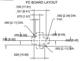
DZ85AB-5-PCB 5 Pin PCB Socket for 40 & 60 Amp Relays - Pins are Included.
